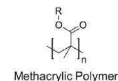
Figure 2. Structure of methacrylic polymer.
