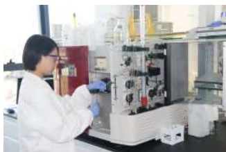
ÄKTA protein purification system - chromatographic performance test
