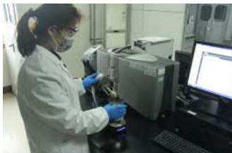
Malvern laser analyzer - particle size analysis
