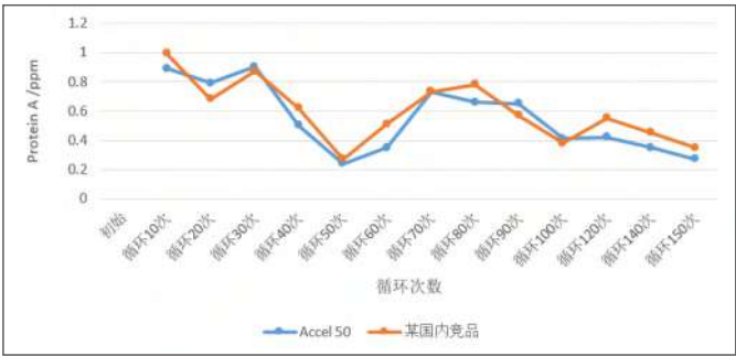
Protein A shedding after 150 cycles of 0.5M NaOH
