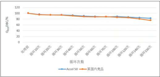
Dynamic capacity retention after 150 cycles of 0.5M NaOH
